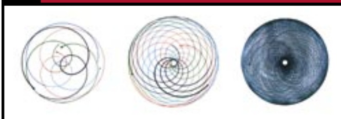
Figure 3. In a double planetary mixer, the orbital motion of blades is both predictable and efficient.
